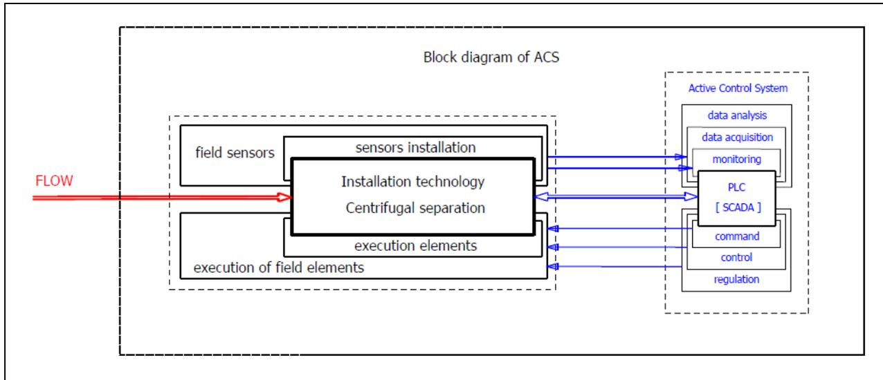
**Fig. 5.8 Block diagram of command and control system.**
