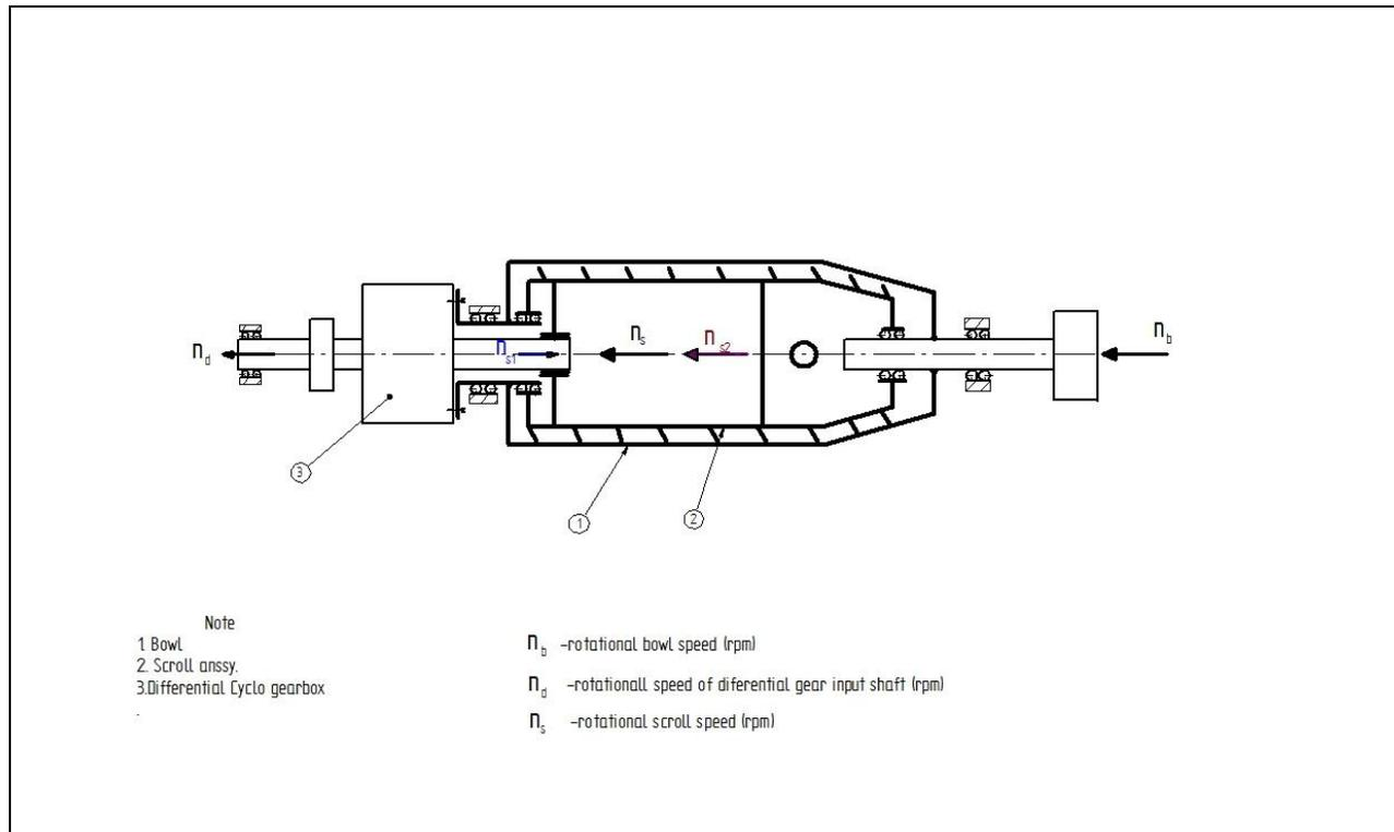
**Fig 5.7 The kinematic scheme of centrifugal separation plant**
