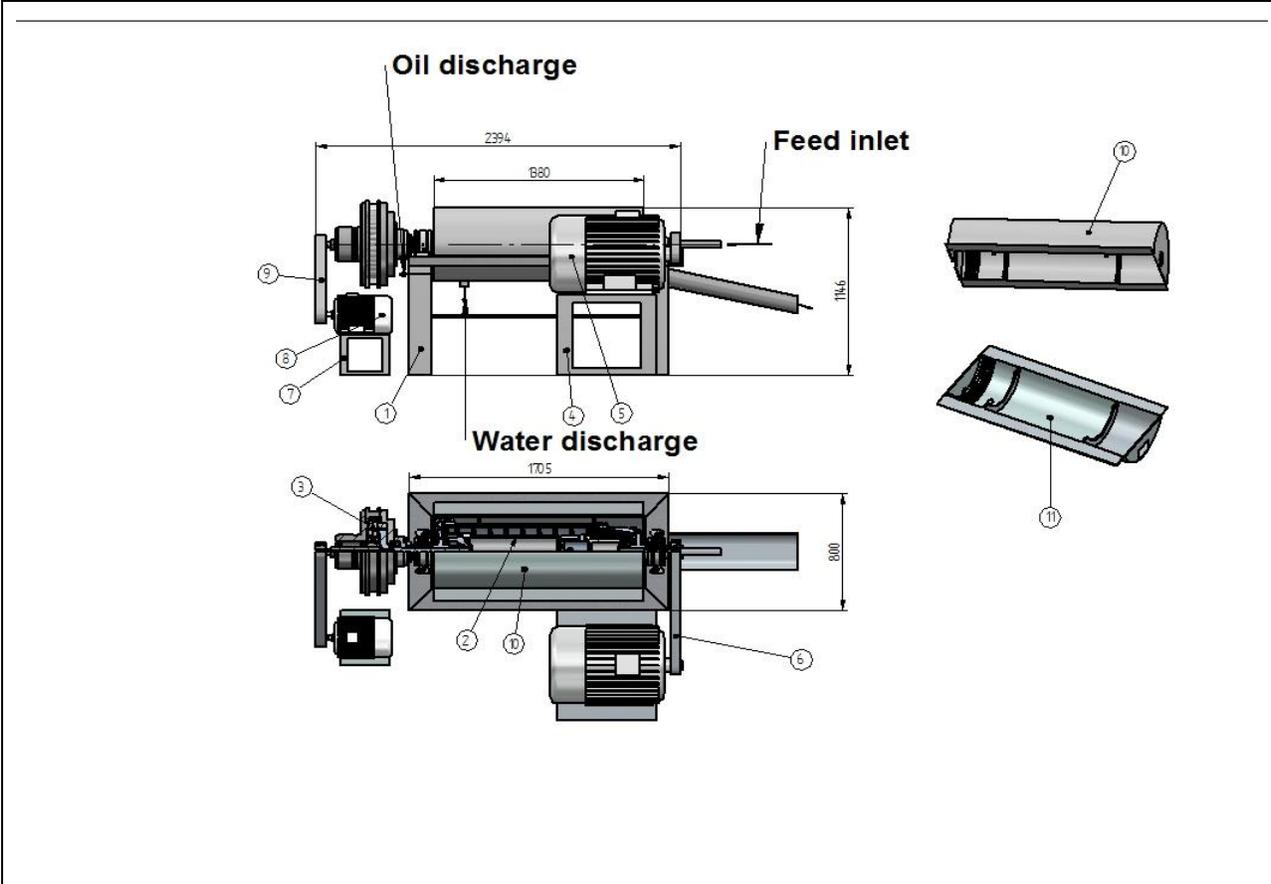
**Fig. 5.5 Overall design of centrifugal separator plant**
