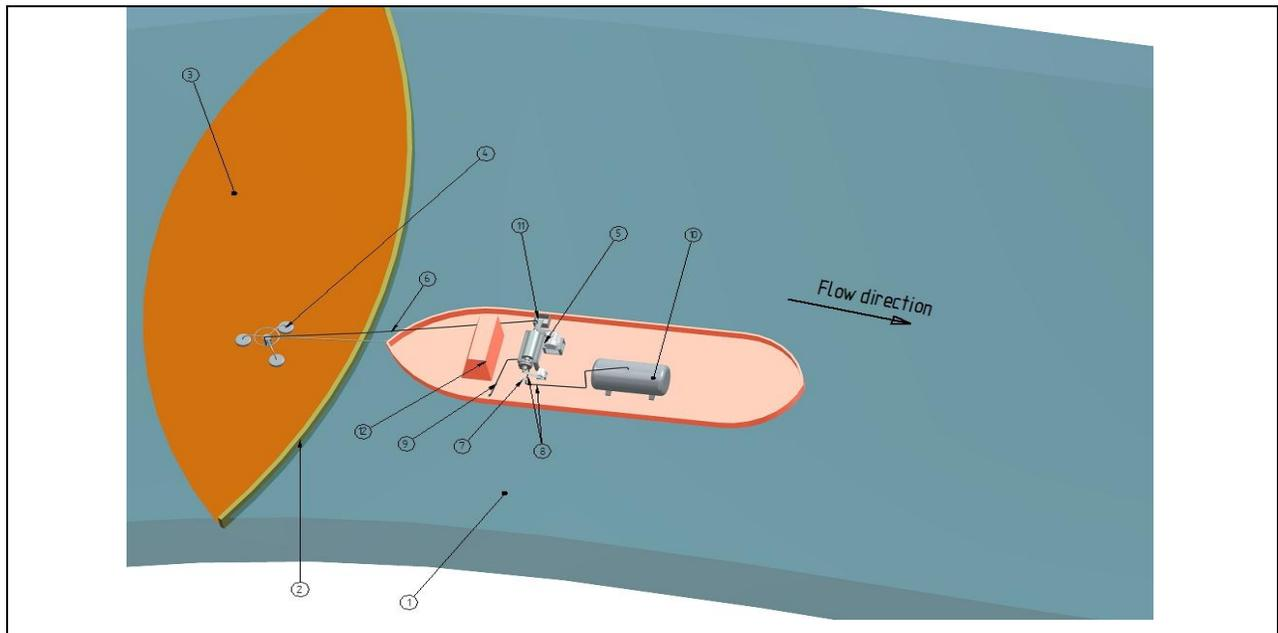
Fig. 5.1 Overview of an ship-mounted installation for the recovery of petroleum products spilled in the waters of the Danube.
