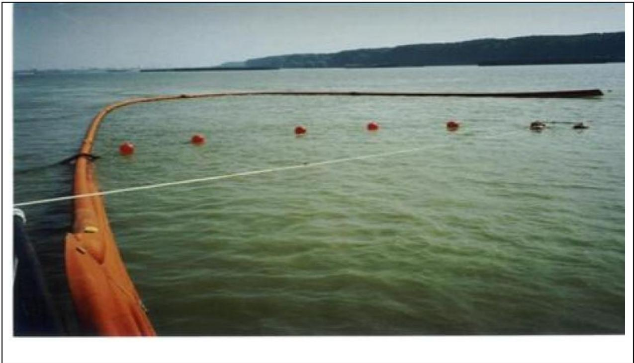
**Fig. 5.1 Inflatable type OIL - BOOM dam**
