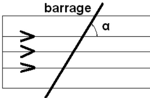
The figure show the setup of a barrage at an angle  $\alpha$  to the current lines. As the current speed increases with both the value of angle diminishes, and the lenght of the barrage go bigger.
