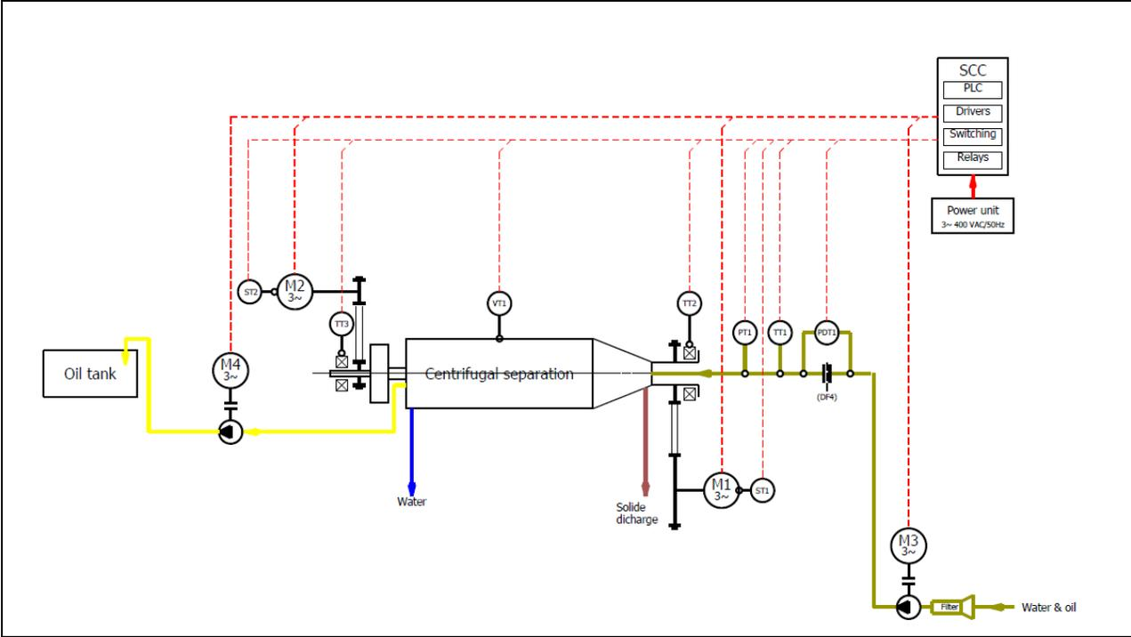
**Fig. 5.9 Instrumentation technological scheme of the installati**
