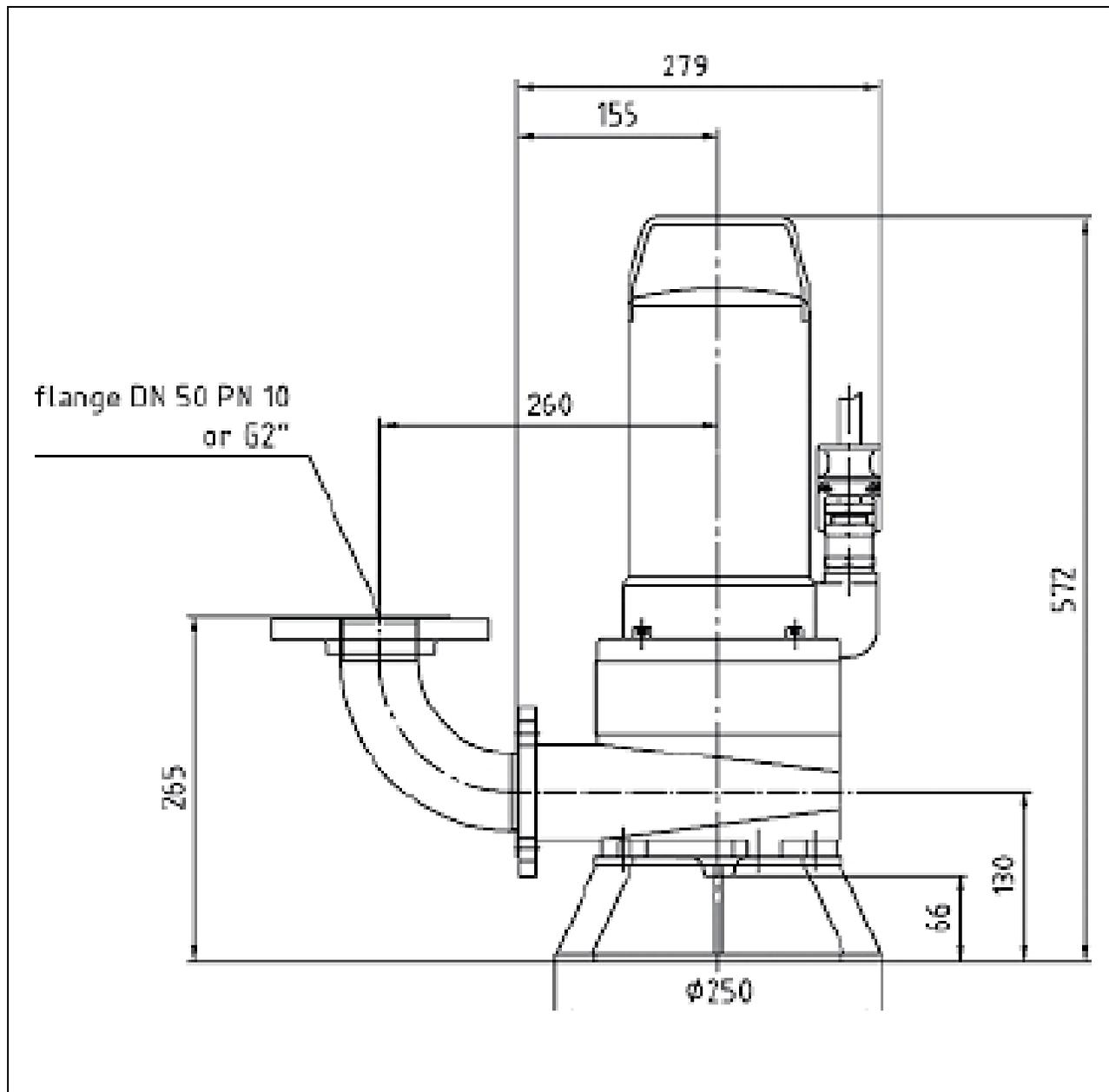
**Fig. 5.4 Overall dimensions of pump ZFS D Ex 70.**
