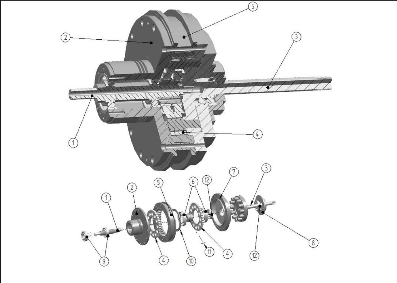
**Fig. 5.6 Cycloidal gearbox**
