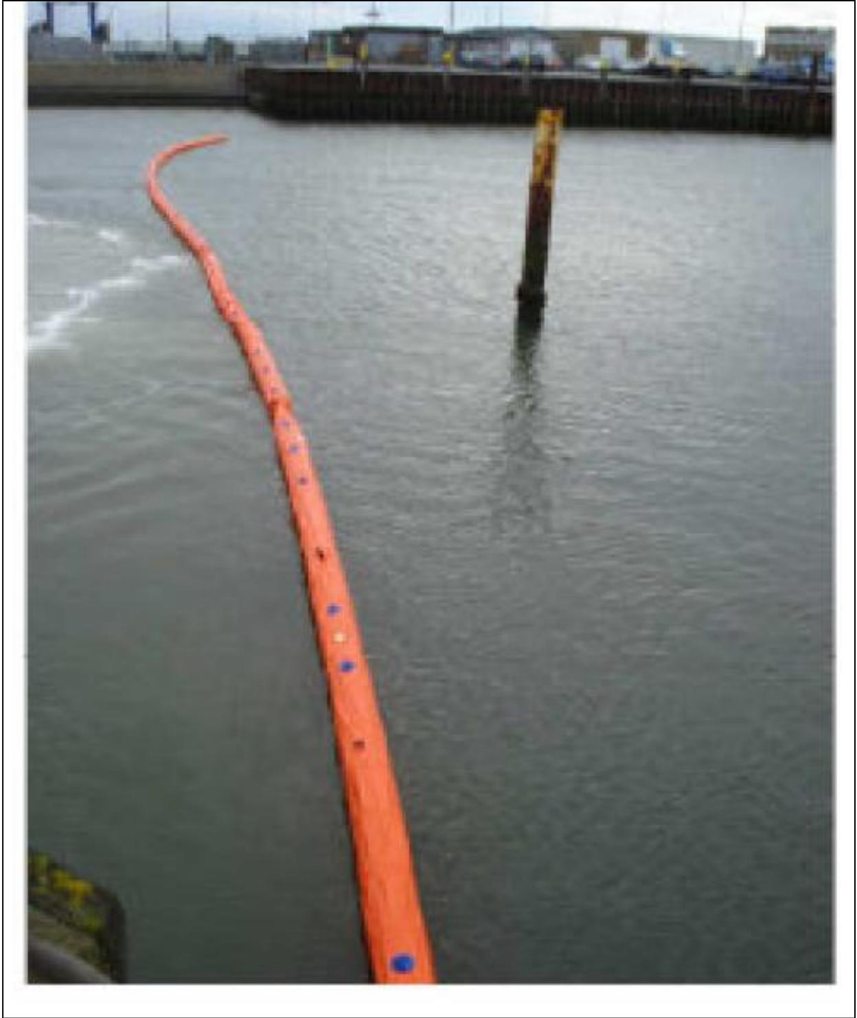
**Fig 5.2 Inflatable type SI- Boom dam**
