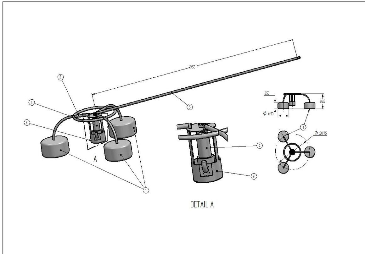
**Fig 5.3 Infested water collection system**
