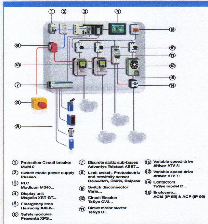
**Fig. 5.10 Establishment of automation and control system structure**
